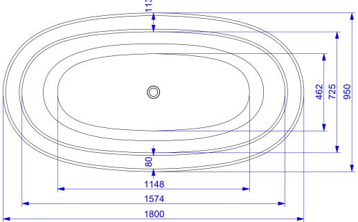
Also available as non-overflowing model Adam-NO. Please follow all local plumbing codes to prepare your bathroom floor for the installation of a non-overflowing bathtub. Specifically - ensure that a floor drain is installed and a proper floor sloping towards the floor drain is observed to eliminate any risk of flooding.
